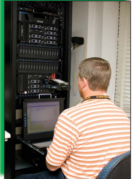
Above: Computer Evidence Recovery Specialist Jeff Knauer previews digital evidence from a computer-related investigation using "Fred", a forensic recovery and extraction device.
