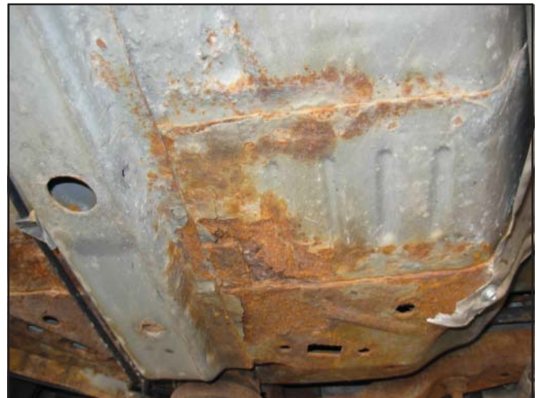
Rust damage on the undercarriage of a squad car.
